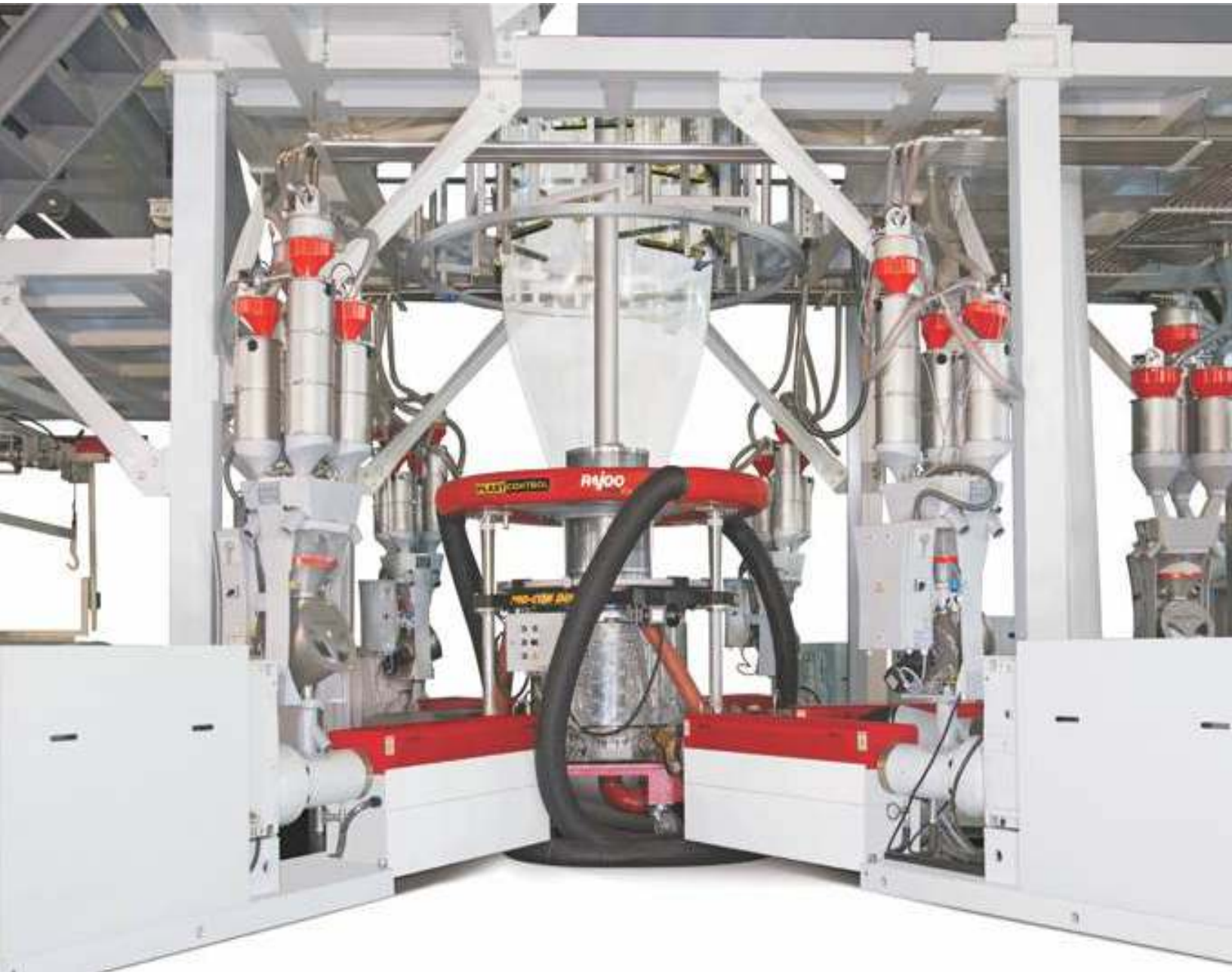
The Pentafoil five-layer co-extruded blown film line
